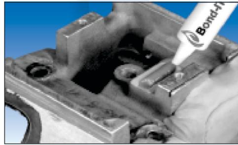
Bond-IT 7056AL Fills a Casting Before Re-Machining
